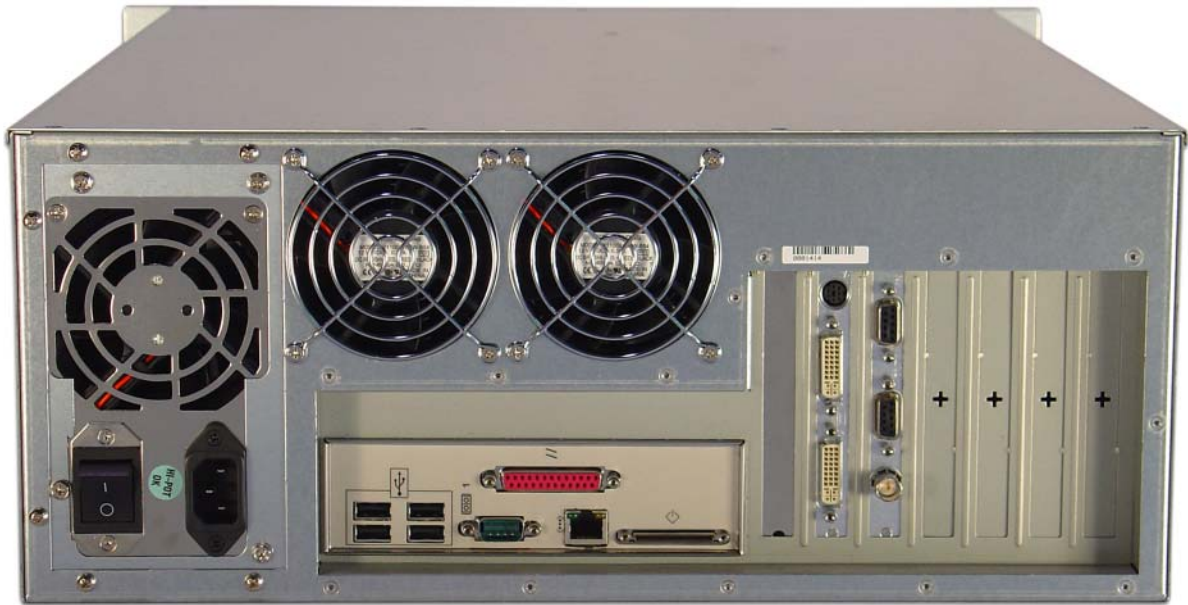
Figure 1 SX2500 Motherboard I/O
